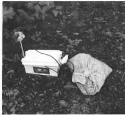
Figure 2. Left. Installing triaxial geophone in ground.
