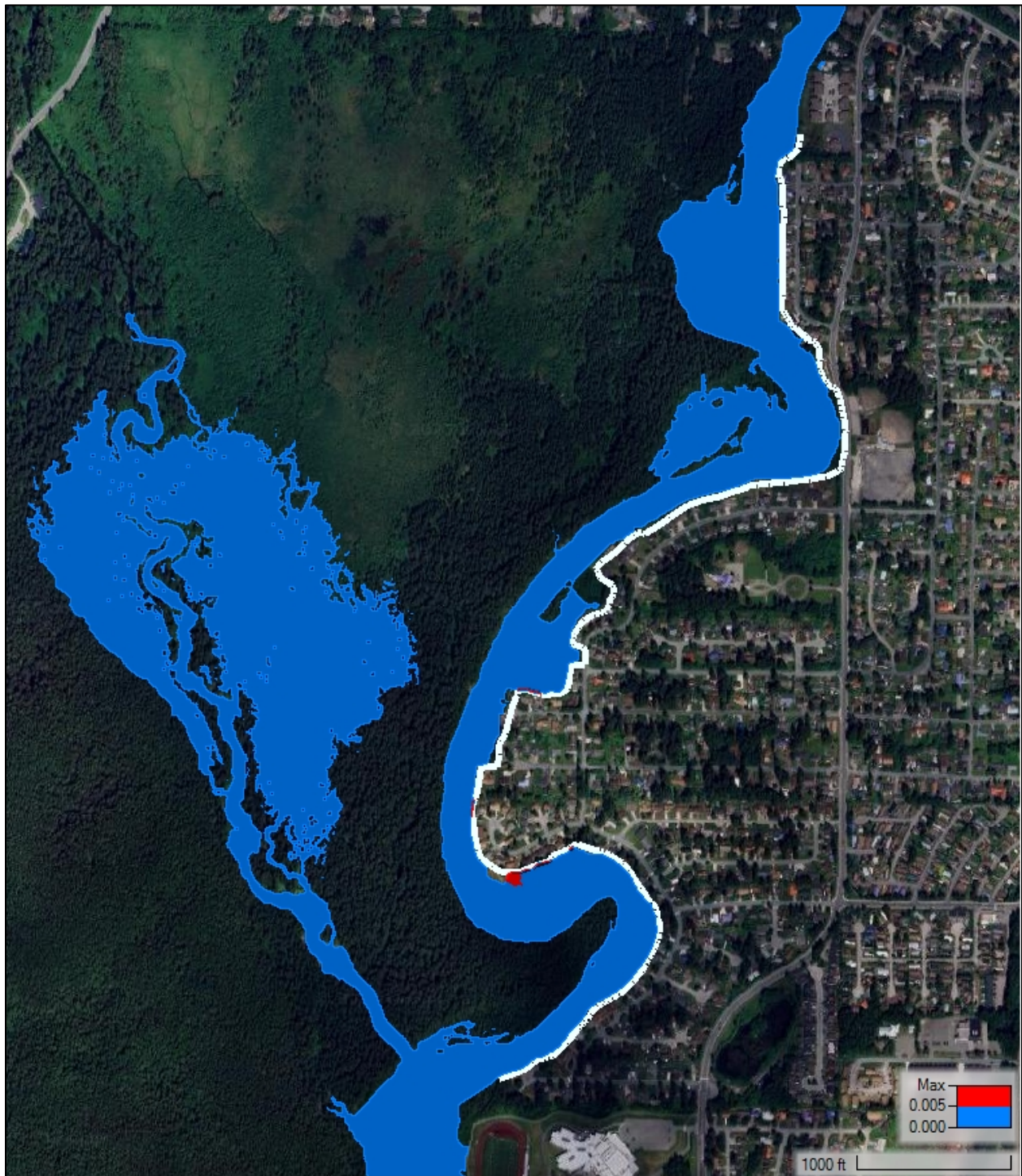
Figure 4-2 Localized rise in 100-Year flood stage (red) as a result of the Proposed HESCO Barrier (white line)
