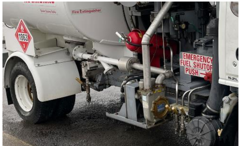
Coastal mobile fueler outfitted with bonding cable, chocked wheels, and emergency fuel shut-off
