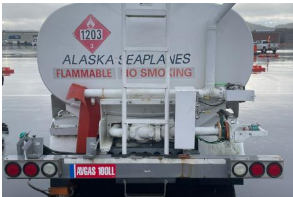
Faded & obstructed placards, Alaska Seaplanes (left) and Ward Air (right)
