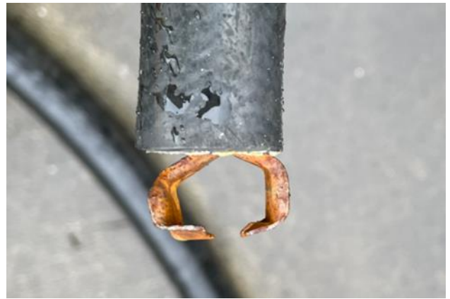
Ward Air emergency fuel shut-off well within the probable spill area (left) and defective bonding cable clip (right)
