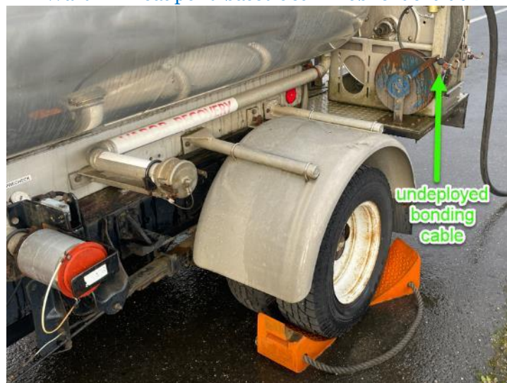
Ward Air fuel truck with undeployed bonding cable
