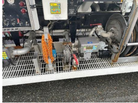
Aero Service Jet A mobile fueler parked on the ramp, properly chocked wheels, placards with good visibility, deadman control (orange cable), and bonding cable on reel
