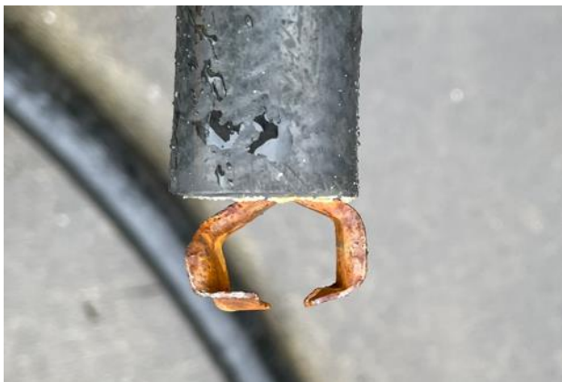
Ward Air Bonding cable clip does not close, the exact condition observed in 2022 and 2023
