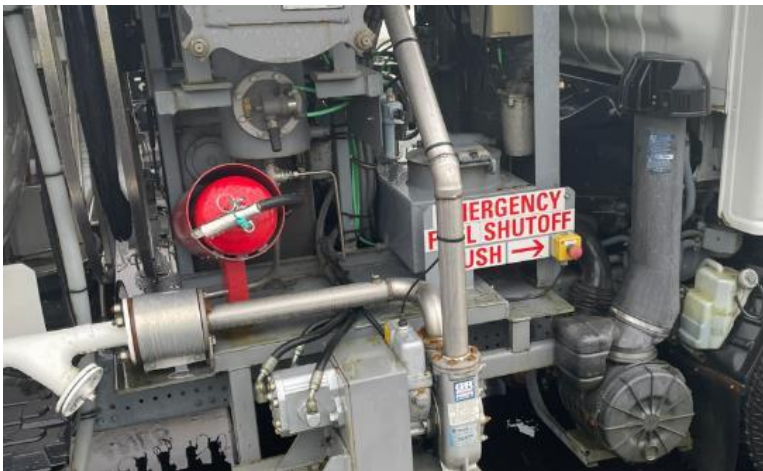
Emergency fuel shut-off button, fire extinguisher, and bonding cable
