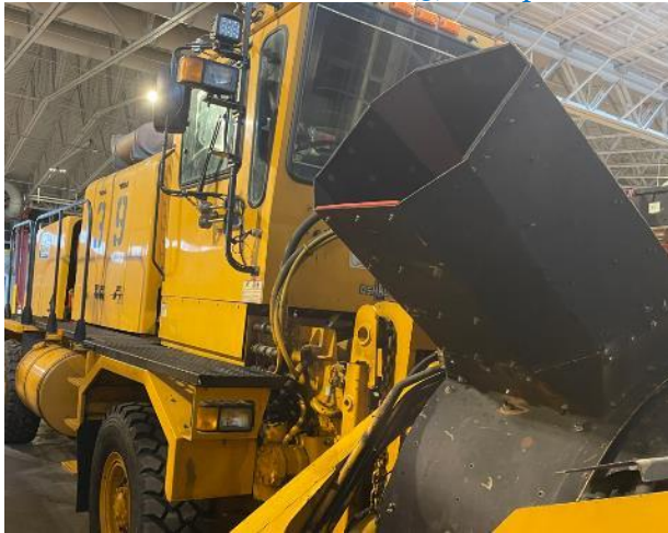
Multi-function machines (3) with plow blade, broom, and blower, the same for all three machines
