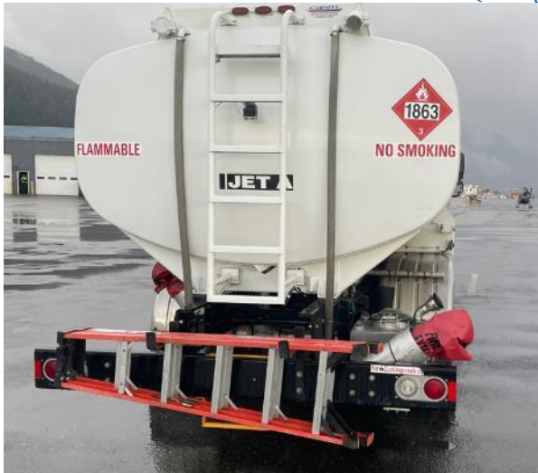
The Jet A mobile fuel truck is outfitted with overfill protection connections, the Jet A placard is partially obstructed (right)
