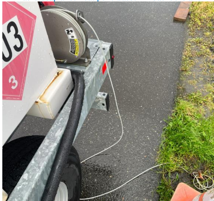
Alaska Seaplanes Av Gas fuel trailer bonding cable clipped to a ground post
