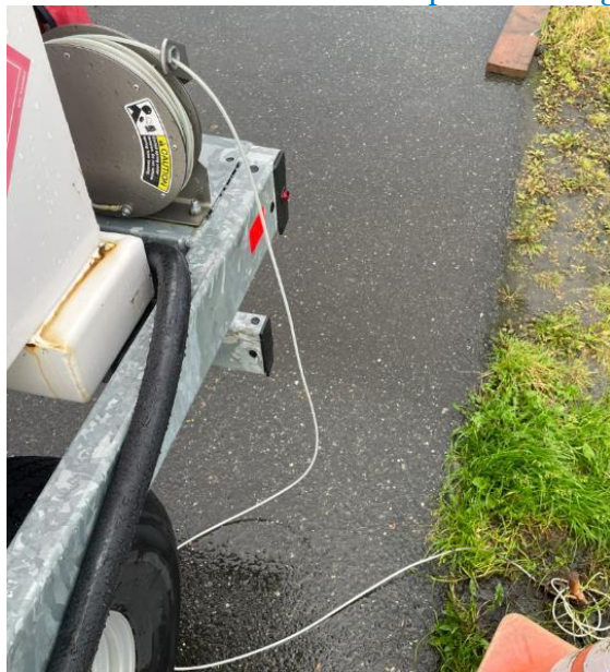
The bonding cable was clipped to a ground post
