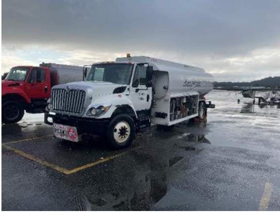
Aero Service Jet A mobile fueler parked on the ramp, properly chocked wheels, placards with good visibility, deadman control (orange cable), and bonding cable on reel
