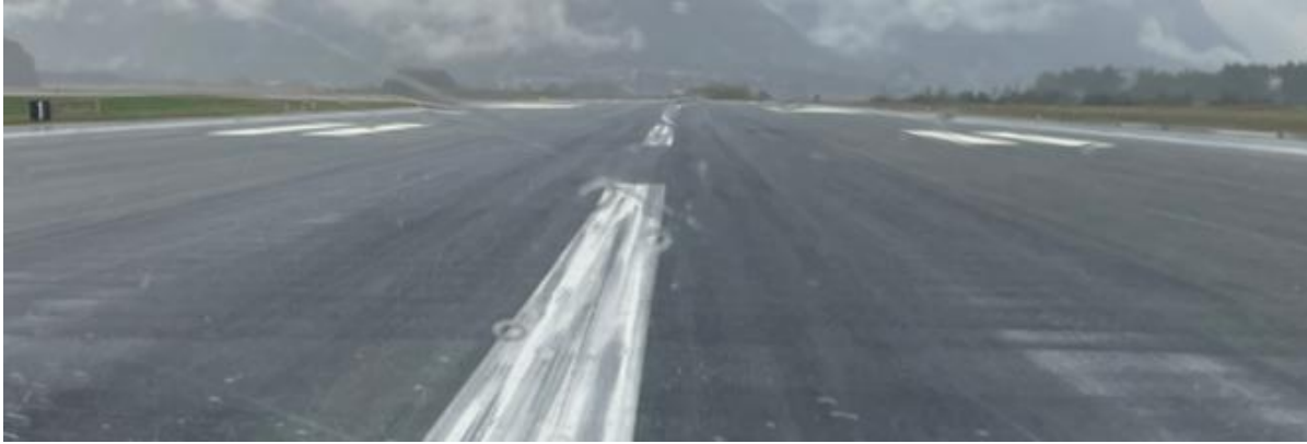
Runway 8 centerline has some rubber build-up
