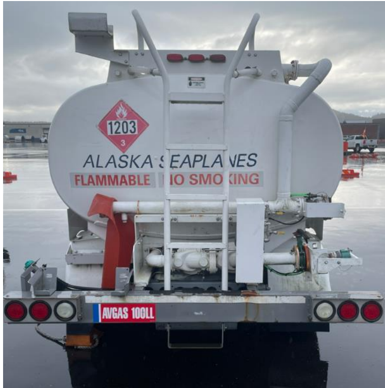
Faded placards “Flammable” & “No Smoking” which is also partially obstructed by the ladder
