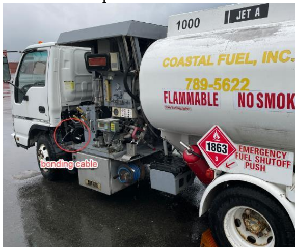
Coastal mobile fueler outfitted with bonding cable, chocked wheels, and emergency fuel shut-off
