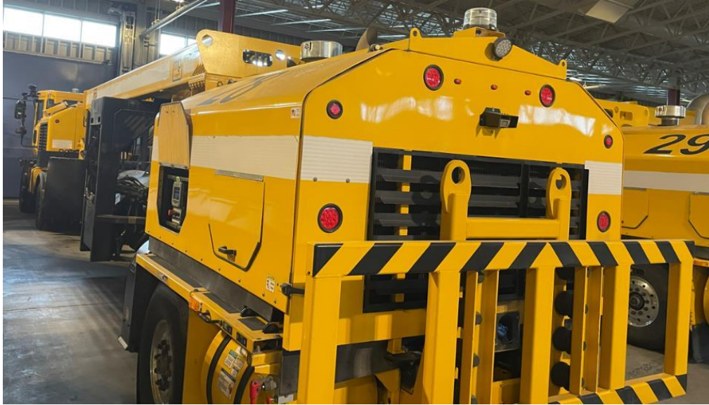
Multi-function machines (3) with plow blade, broom, and blower, the same for all three machines
