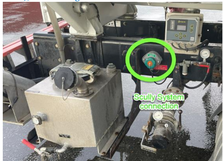
The Jet A mobile fuel truck is outfitted with overfill protection connections, the Jet A placard is partially obstructed (right)
