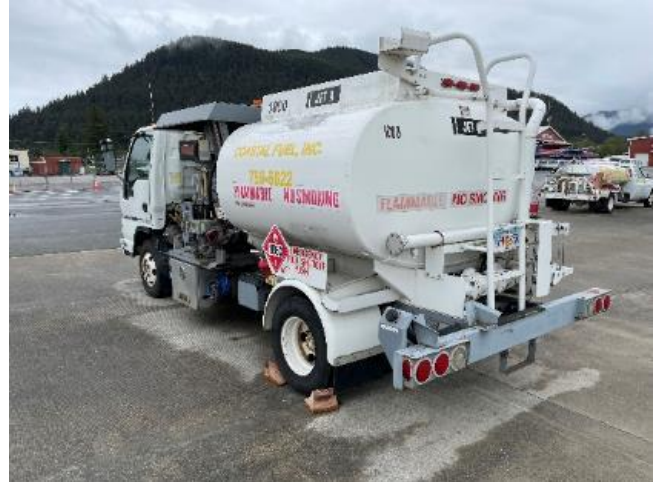
Jet A mobile fuel truck, faded placards should be replaced, wheels properly chocked
