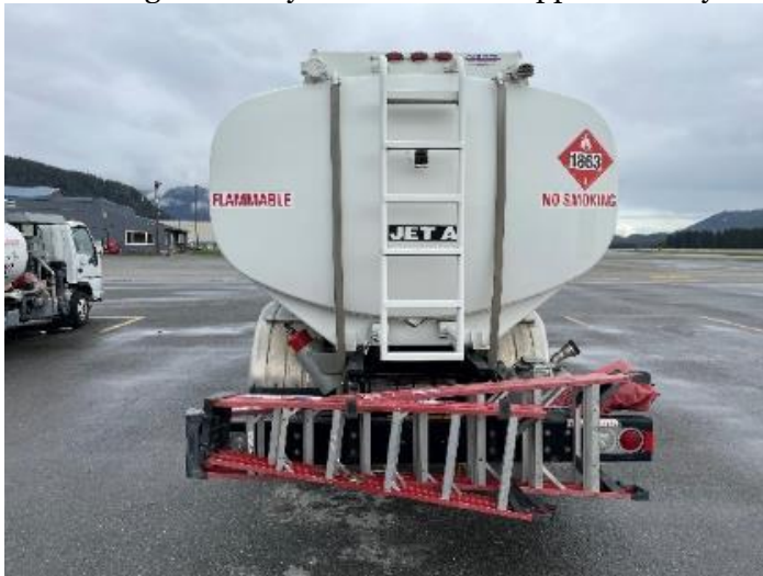
Aero Service Jet A mobile fueler parked on the ramp, properly chocked wheels, placards with good visibility
