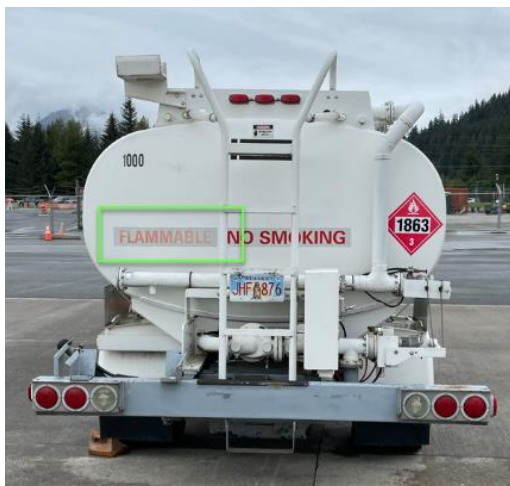
Coastal mobile fuel trucks with isolated faded placards (Flammable & No Smoking), faded emergency fuel shut-off button
