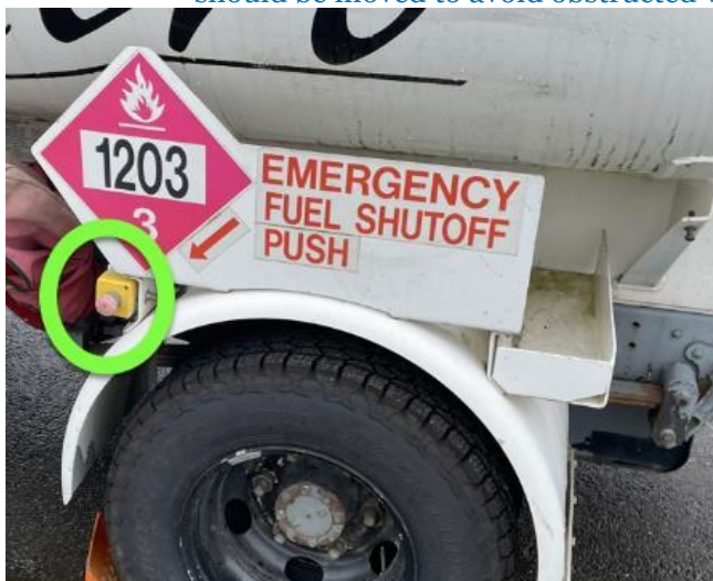
The emergency fuel shut-off button was faded, so it should be re-painted bright red, the bonding cable was in good condition
