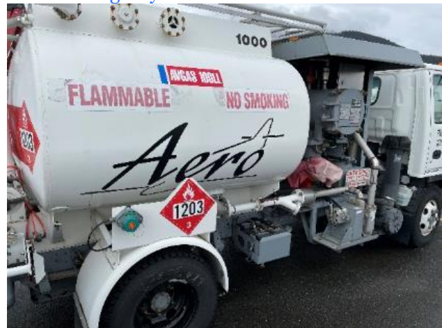
Av Gas mobile fuel truck has faded placards in need of replacement (No Smoking & Flammable), the rear placards should be moved to avoid obstructed view from the fixed & step ladders
