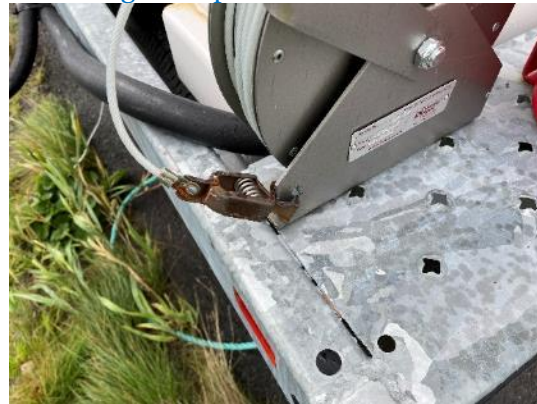
Ramp to dock (left), bonding cable coiled inside the reel on the fuel trailer
