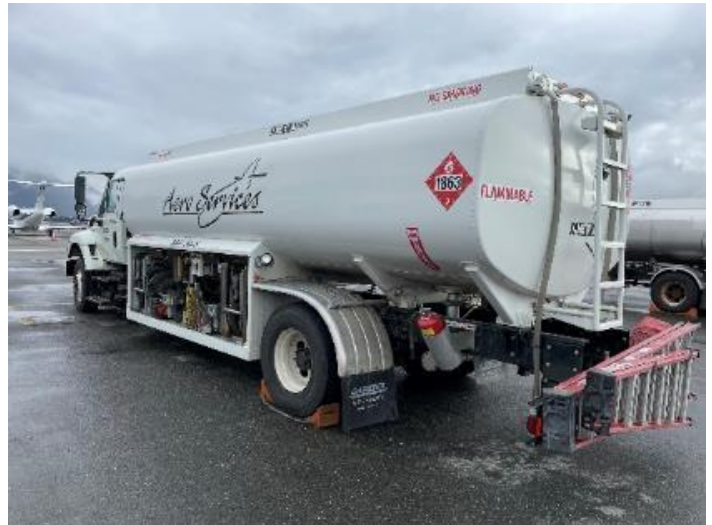
Aero Service Jet A mobile fueler parked on the ramp, properly chocked wheels, placards with good visibility
