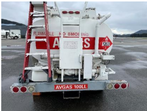
Av Gas mobile fuel truck has faded placards in need of replacement (No Smoking & Flammable), the rear placards should be moved to avoid obstructed view from the fixed & step ladders
