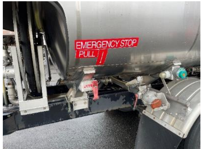
The Jet A mobile fuel truck is outfitted with overfill protection connections and clearly visible emergency fuel shut-off lever, however signage should state "Emergency Fuel Shut Off."
