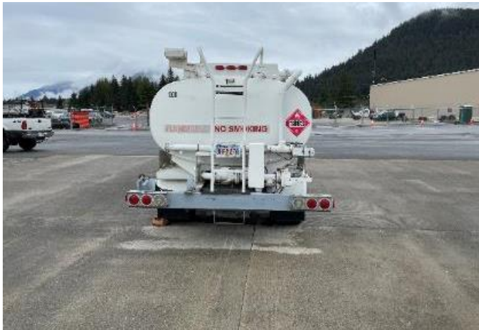
Jet A mobile fuel truck, faded placards should be replaced, wheels properly chocked
