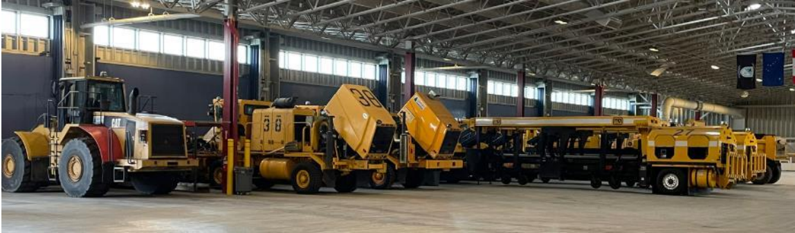
Multi-function machines (3) with plow blade, broom, and blower, the same for all three machines
