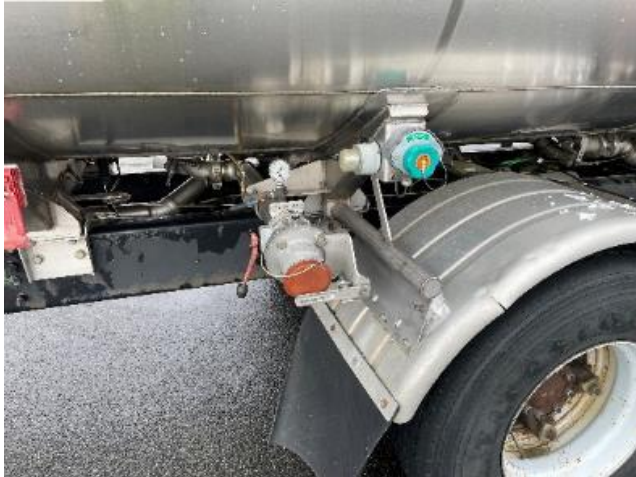
The Jet A mobile fuel truck is outfitted with overfill protection connections and clearly visible emergency fuel shut-off lever, however signage should state "Emergency Fuel Shut Off."
