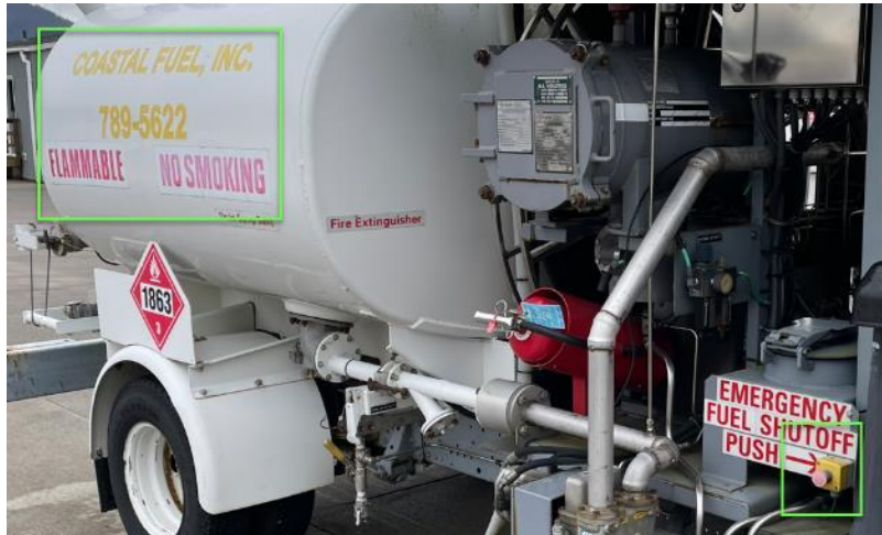
Coastal mobile fuel trucks with isolated faded placards (Flammable & No Smoking), faded emergency fuel shut-off button
