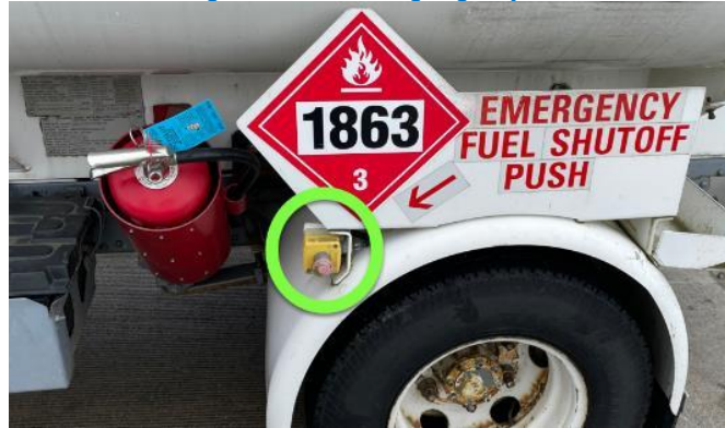
Bonding cable/clip in good condition, the emergency fuel shut-off button is faded and should be painted bright red to restore high visibility appearance
