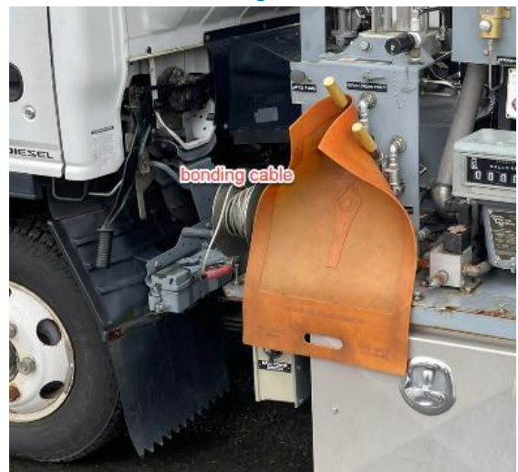
The emergency fuel shut-off button was faded, so it should be re-painted bright red, the bonding cable was in good condition
