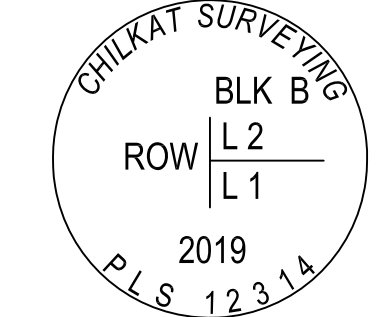
TYPICAL MONUMENT DETAIL N.T.S. 5/8" x 3/8" REBAR WITH 2.5" ALUMINUM CAP
