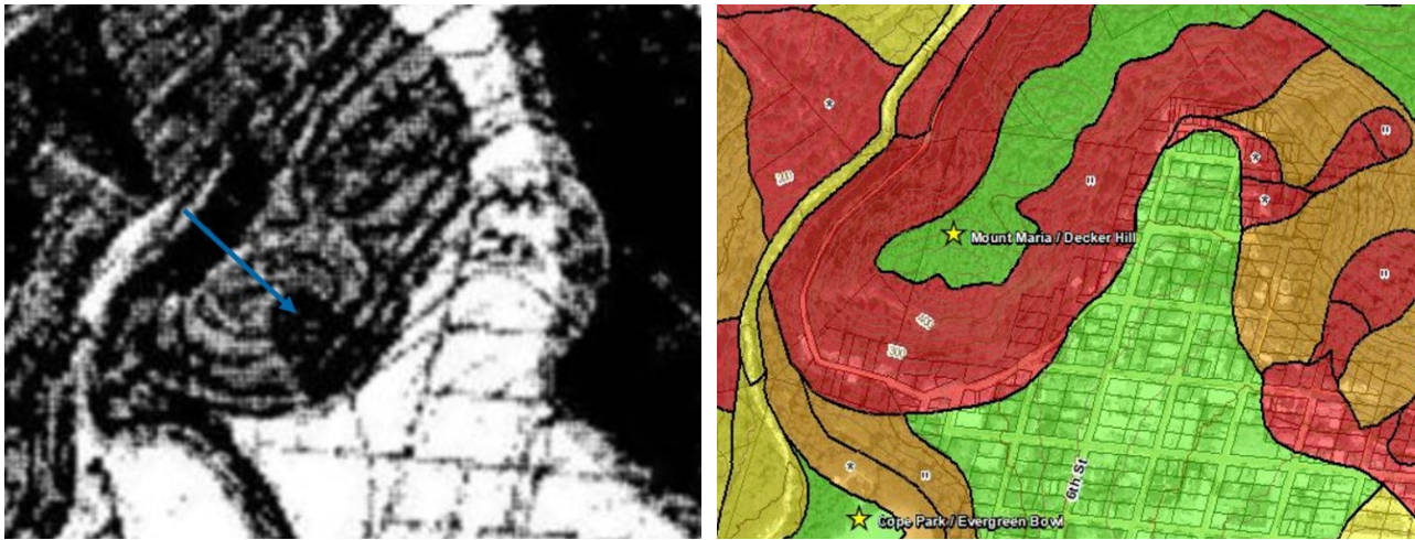
Figure 4: Comparison of Swanston's Figure 6 (left) and Tetra Tech's Figures 1.6c and 1.6h Landslide Hazard Designation Mapping (right). Swanston (1972) uses Potential Hazard (gray) and High Hazard (black), designated in the 1987 adopted mapping as Moderate and Severe hazards. Tetra Tech uses Low (green), Moderate (yellow), High (orange) and Severe (red) hazard designations.
