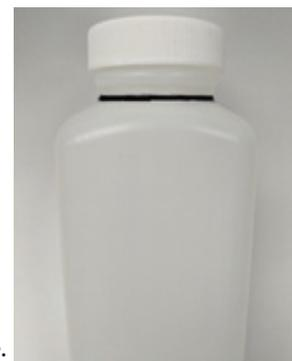
Both the empty Reagent Water container and the filled Field Blank container must be returned to the lab along with the samples taken.
