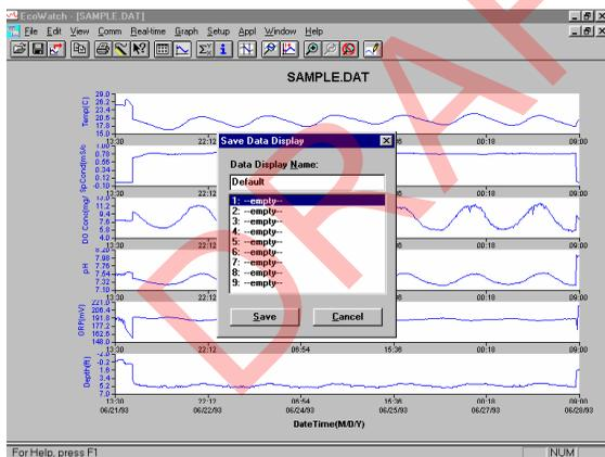
Then type “Default” for the file name and click **Save**. The parameters, colors, format, and x-axis time interval associated with the current display are now saved and can be accessed any time in the future. Nine different data displays may be saved for any data file. You can easily switch between various displays of the data. The data files can be accessed by clicking **Load Data Display** from the file menu and then selecting the desired presentation.
