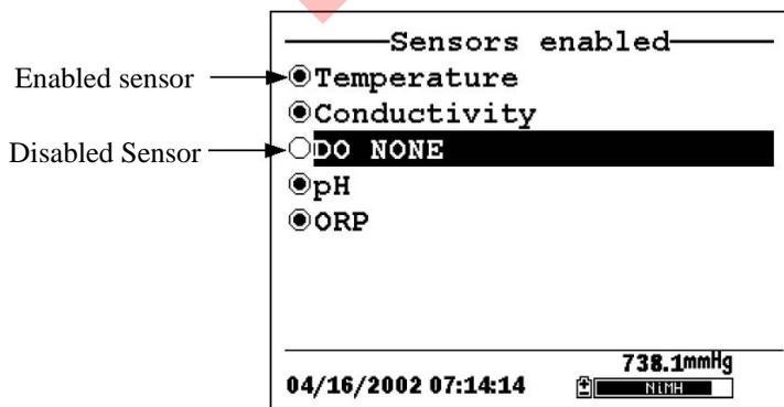
**Figure 4.2 Sensors Enabled Screen Before DO Membrane Selection**
