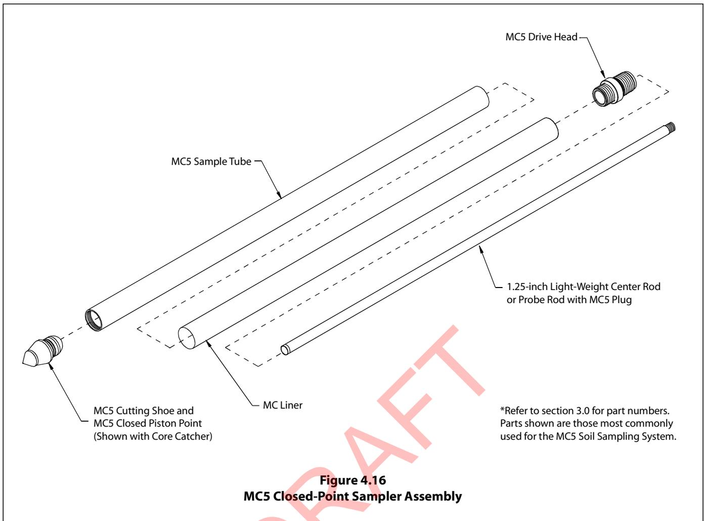
7. Thread an MC5 Plug (23641) onto 1.25-inch light-weight center rod (Fig.4.22). Note that light-weight center rods are only available in 48-inch and 60-inch lengths. Utilize 1.25-inch probe rods if other lengths are required.
