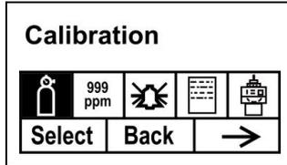
Select Zero or Span Calibration by pressing [N/+]. Once your choice is highlighted, press [Y/+].
