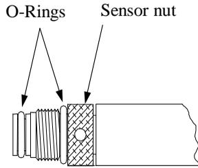
**Figure 3.4 O-ring Lubrication**
