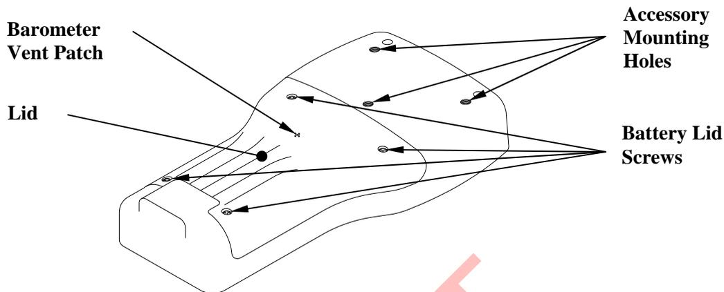
**Figure 2.2 Back View of YSI 556 MPS**
