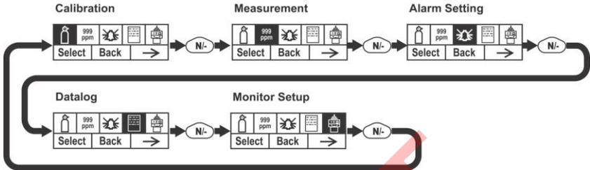
**Note:** When you reach Monitor Setup and press [N/-], the menu cycles back to Calibration.
