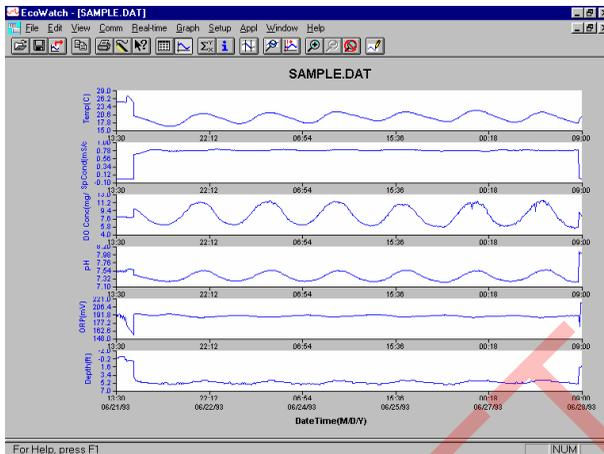
From the **Setup** menu, click **Graph**. Click **2 Traces per Graph** and notice that the parameters are now graphed in pairs for easy comparison of parameters.
