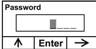
2. In Basic User Level, you do not need a password to perform calibrations. Instead of inputting a password, enter calibration by pressing [MODE].
