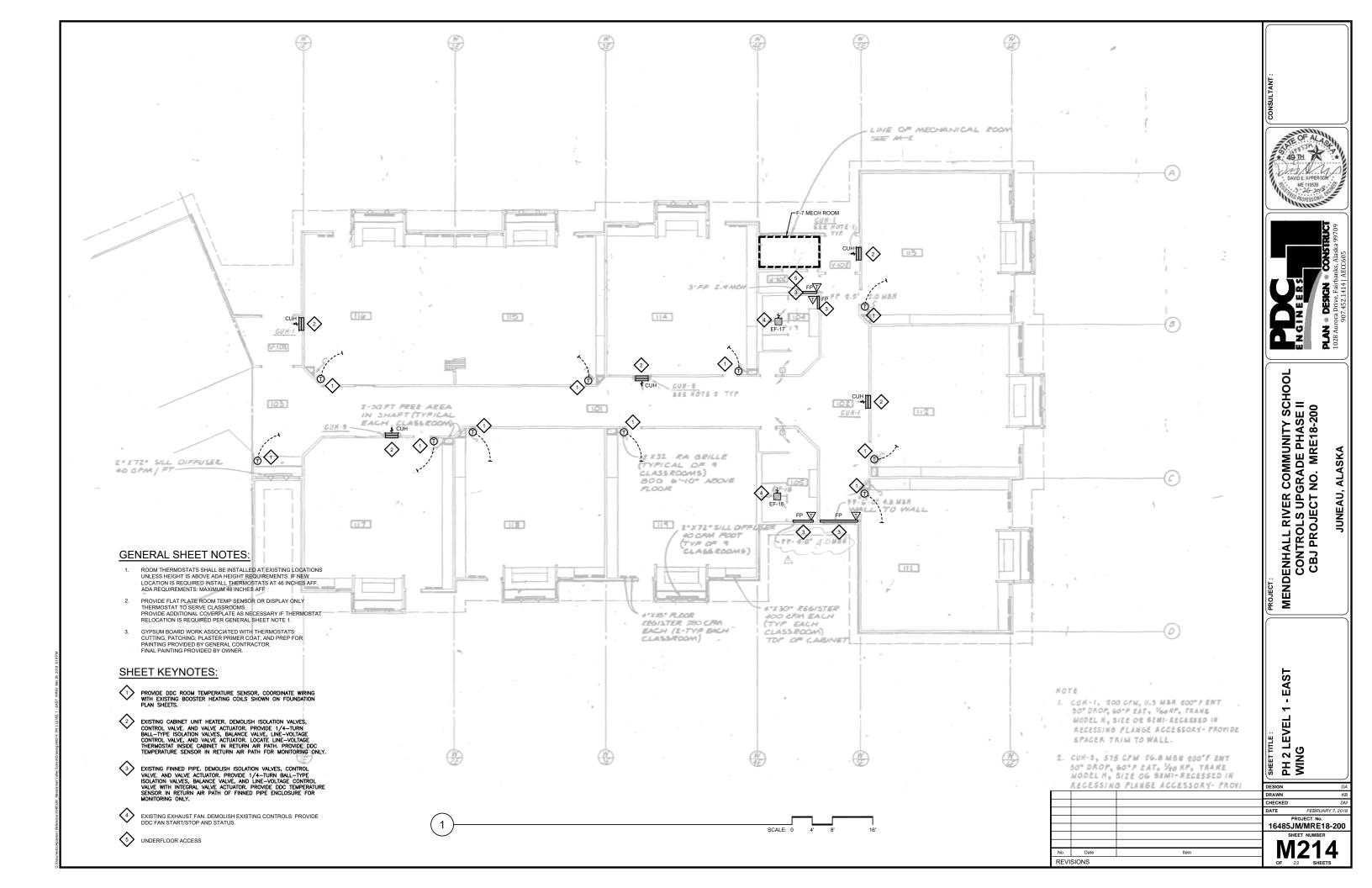
ALL CONTROL VALVES, SENSORS, AND CONTROL DEVICES TO BE NEW, REPLACE EXISTING IF APPLICABLE. MOTORS, & FANS ARE EXISTING TO REMAIN. SEE SEQUENCE OF OPERATION. PROVIDE CURRENT SENSORS FOR MONITORING AS SPECIFIED TO MOTORS AND FANS.
