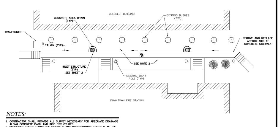
2. DISTURBED AREAS ALONG THE SIDEWALK AND CONSTRUCTION AREAS SHALL BE RETURNED TO ORIGINAL OR BETTER CONDITION.
