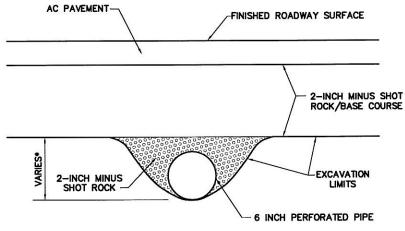
\*ADJUST DEPTH AS REQUIRED TO MAINTAIN 1% MINIMUM GRADIENT
