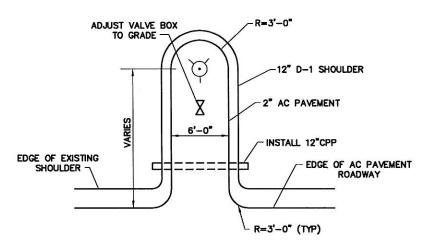
CONSTRUCT HYDRANT ACCESS PAD WITH USABLE EXCAVATION AS NECESSARY, 4 INCHES BASE COURSE, GRADING D-1 AND 2" AC PAVEMENT.
