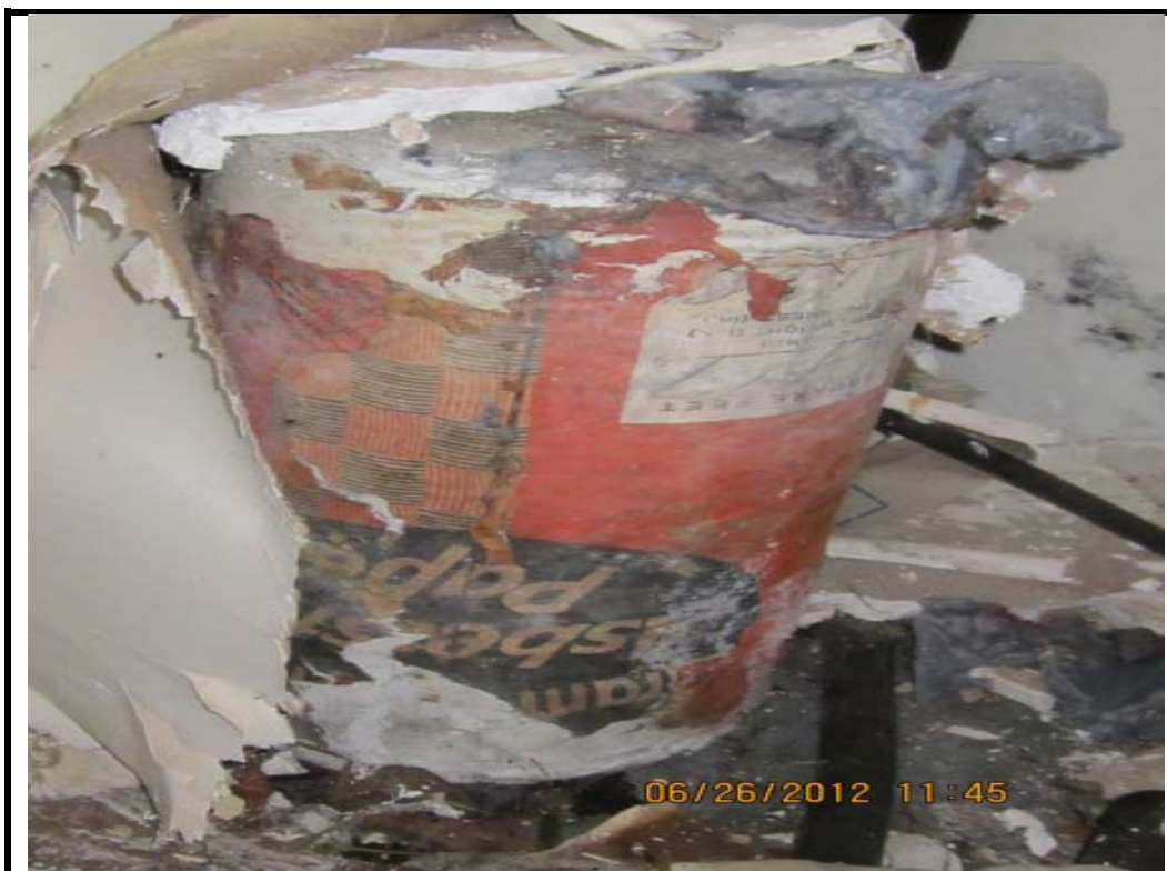
Photo 14: Hazardous material identified in Room 1. Asbestos paper.
