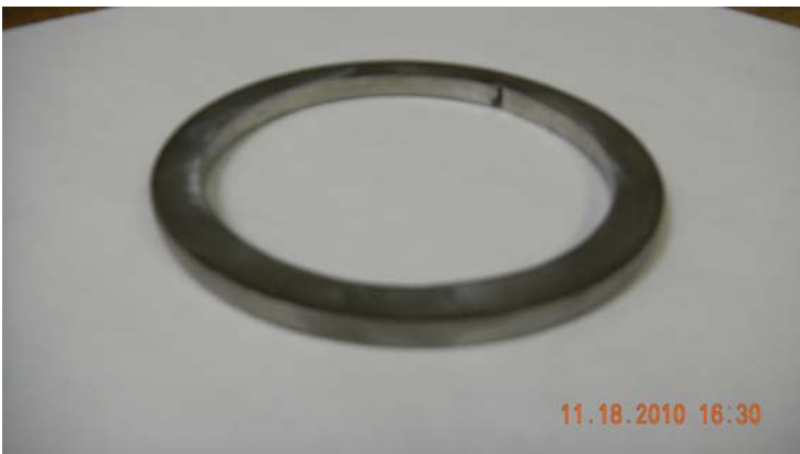
Photo 3: Typical lower end tube repair ring
