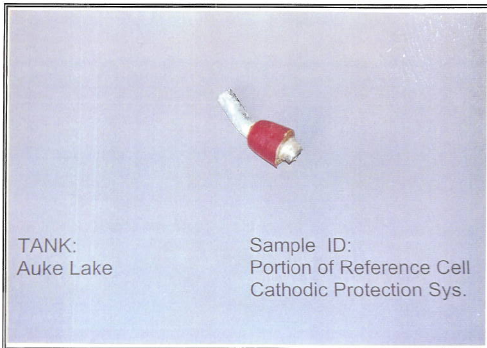
PHOTO No. 11: Cathodic Protection System, Damaged Reference Cell - This portion of the reference cell was found on the tank floor beneath the reference cell location at the Tier C, Bottom Panel, 11:50 position.
