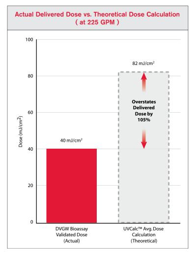
The graph above highlights an actual comparison of DVGW bioassay validation results with theoretical dose calculations using UVCalc™ for a TrojanUVSwift™SC at a flow rate of 225 GPM. The theoretical calculation overstates the delivered dose by 105%. Had a drinking water system been selected based on the results of the calculated dose, public safety could be seriously compromised.
