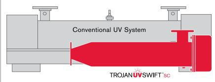
The highly efficient "L-shaped" design and LPHO amalgam lamps result in an extremely compact footprint, as shown in the size comparison with a conventional "U-shaped" low-pressure system – both of which are capable of treating approximately 175 GPM (40 m³/hr) at 90% UVT.
