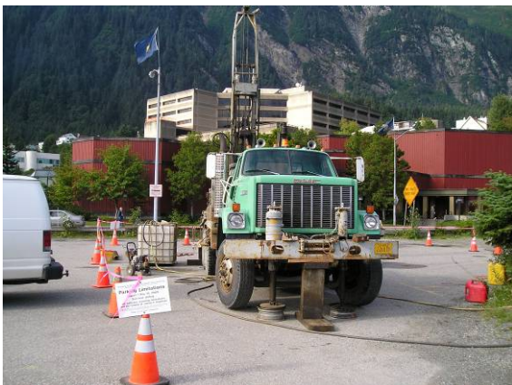
The R&M CME-55 truck mounted drill rig.
