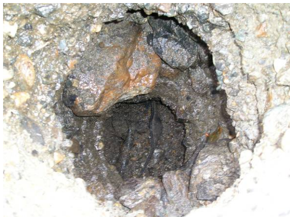
The A-J rockfill layer. In these photos, the voids typically within the rock fill were already filled with drill cuttings and bentonite mud.
