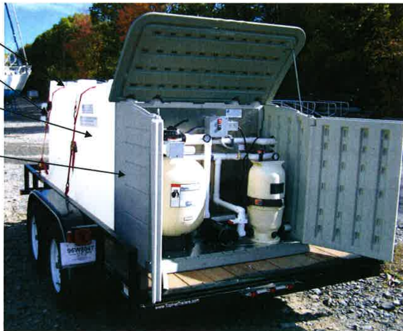
Plastic enclosure for filters, pump, and controls.
