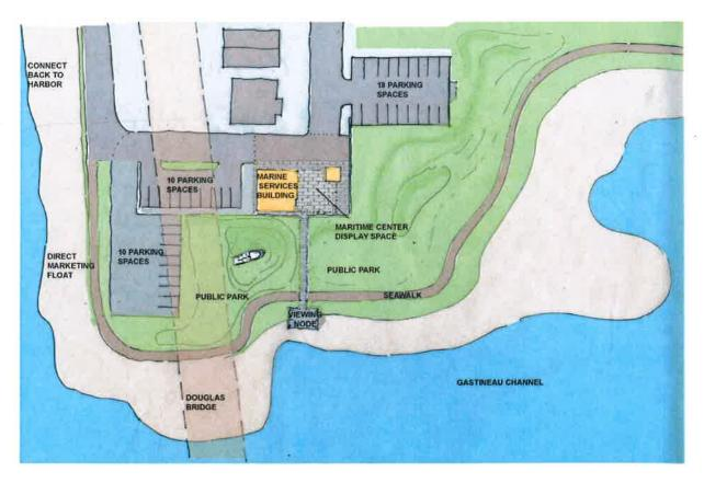
This scheme places the building perpendicular to the bridge and on axis with West 9<sup>th</sup> Street, allowing for the street hardscape to essentially flow through the lobby area and connect with the terminating dock node on the water's edge. This has the strongest connection to the park site; it has the best park to building integration. The public has access all around the building. It has a more formal walkway on the street side and more organic seawalk pathways on the water side.
