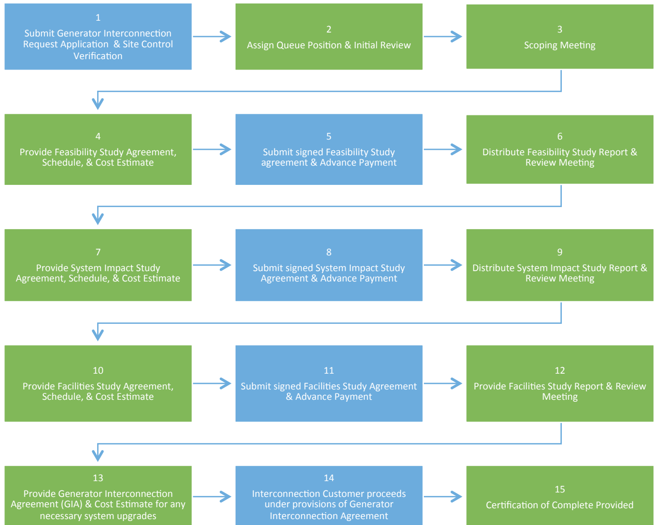
Generator Interconnection Request Flow Chart ( \geq 5,000 kVA)
