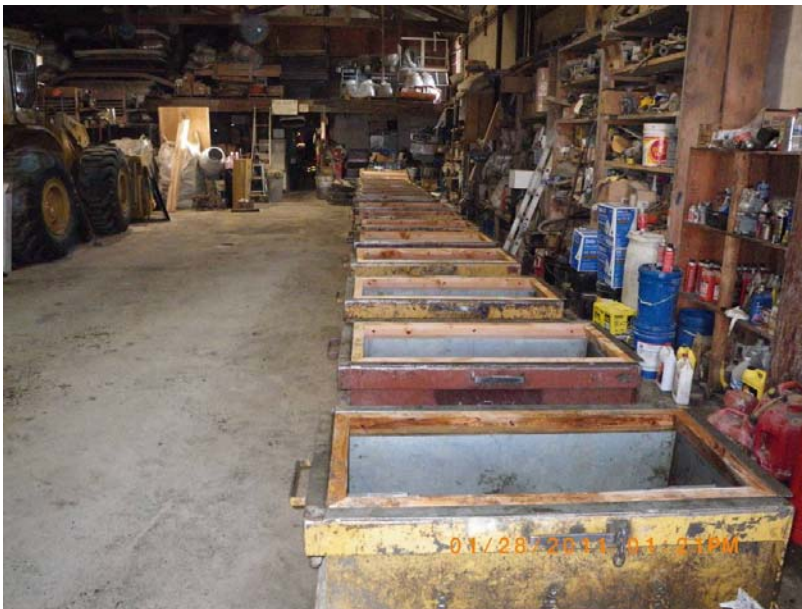
Forms for shoulder blocks for new float plane launch ramps.
