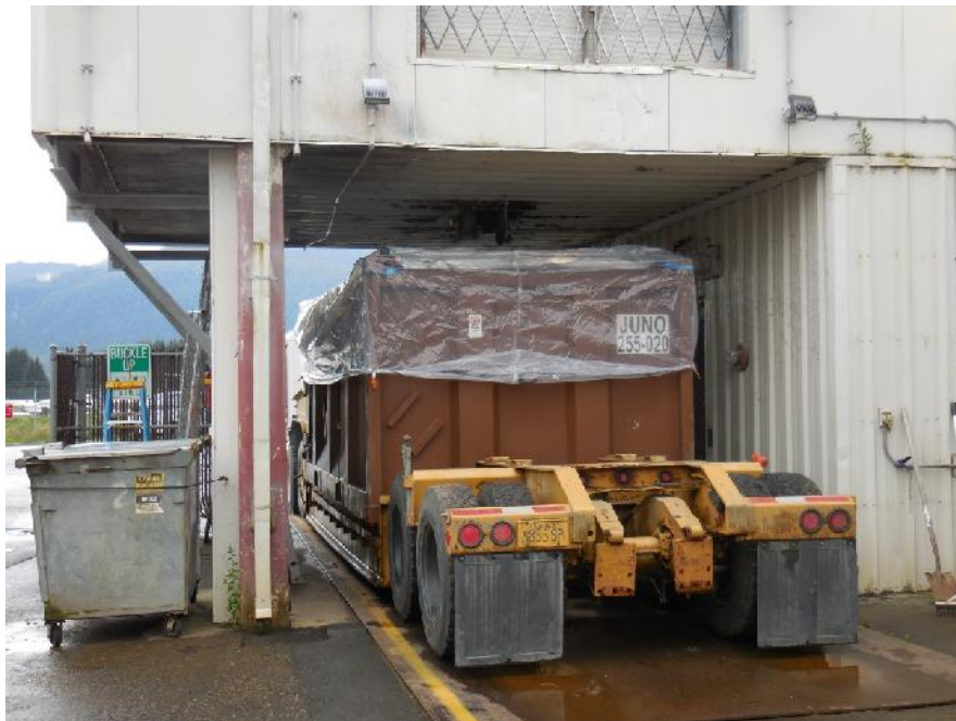
Figure 14. Lined Conex Container on a Low Boy Truck
