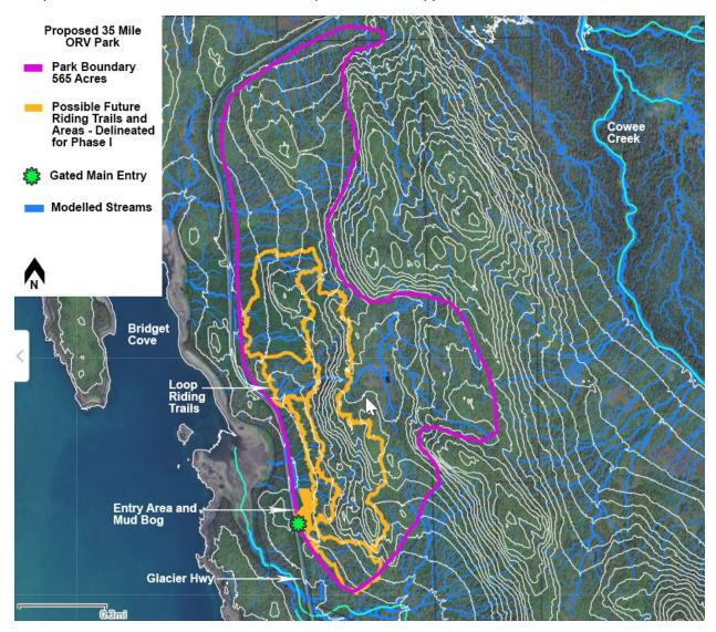
For Phase I, potential trails, parking area and site features are mapped in the field with GPS tracks and shown on the plan. The wetland delineation has been performed and an Army Corps of Engineers permit is being submitted. The proposed park consists of a gated entrance, parking area, picnic area and caretaker facility on an existing upland fill pad, loop riding trails, mud bog, and cross country riding.
