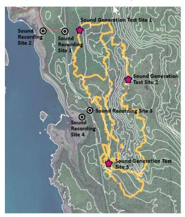
A 4 wheel drive ORV model Can Am Outlander 1000r 976cc V-Twin was started up and ran at 4000 rpm at Sound Generation Test Site 3 by the proposed parking lot where an existing old roadbed allowed access into the site. The other two sound generation sites were more remote and access with an OHV was not possible, at these sites a chainsaw on idle generated similar decibel levels. The sound recording instrument was a Vlike VL6708 Digital Sound Level Meter.
