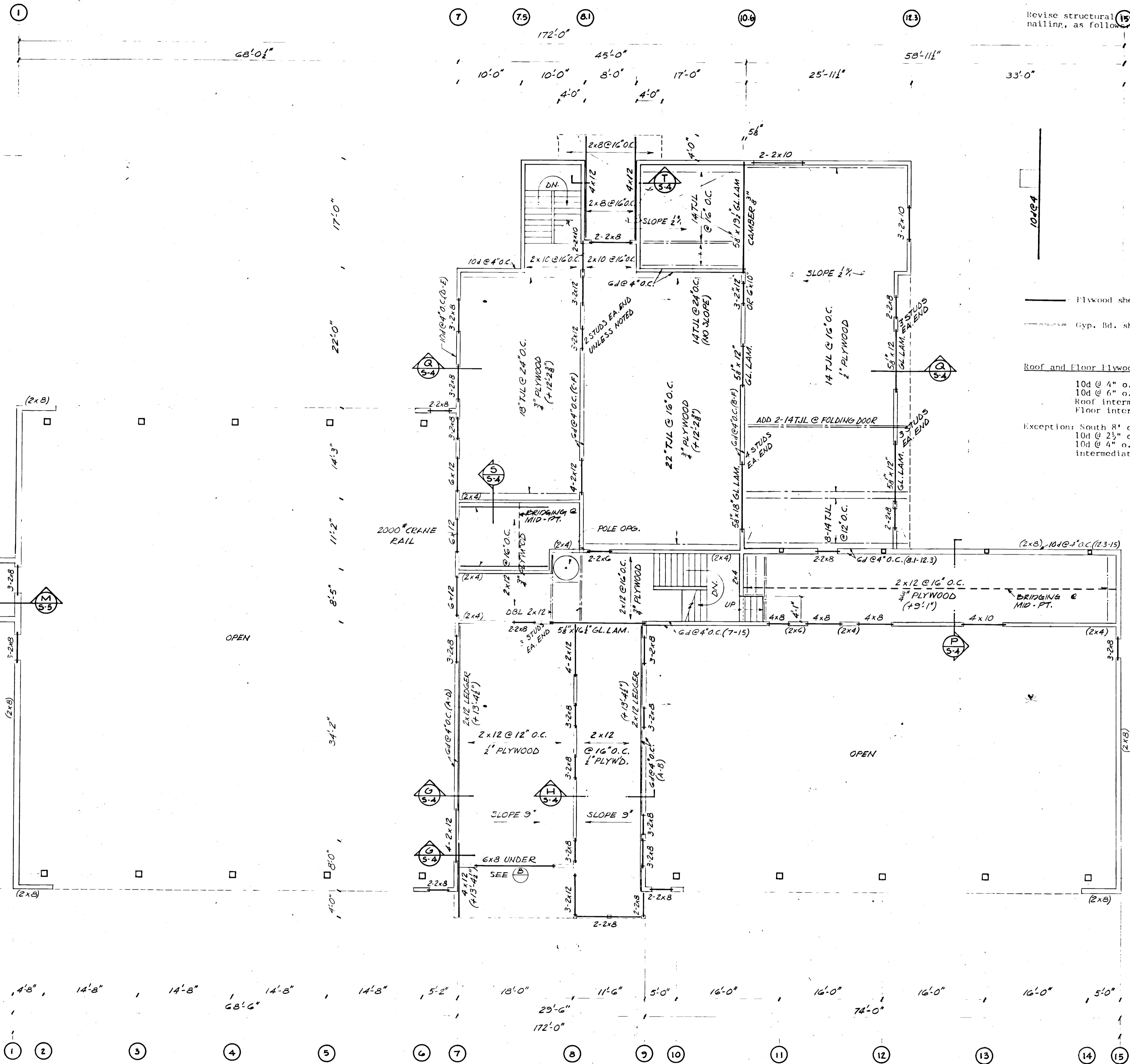
LOW ROOF & 2ND FLOOR FRAMING PLAN 1/8" = 1'-0"
