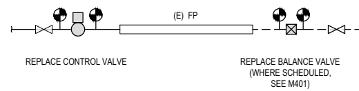
2 Baseboard Heater Piping Diagram
