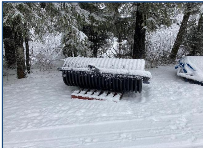
*Figure A1. Roller used for compacting fresh snow.*
