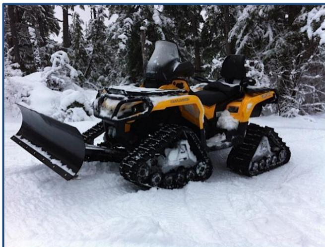
*Figure A3. Can-Am 4-track with plow.*
