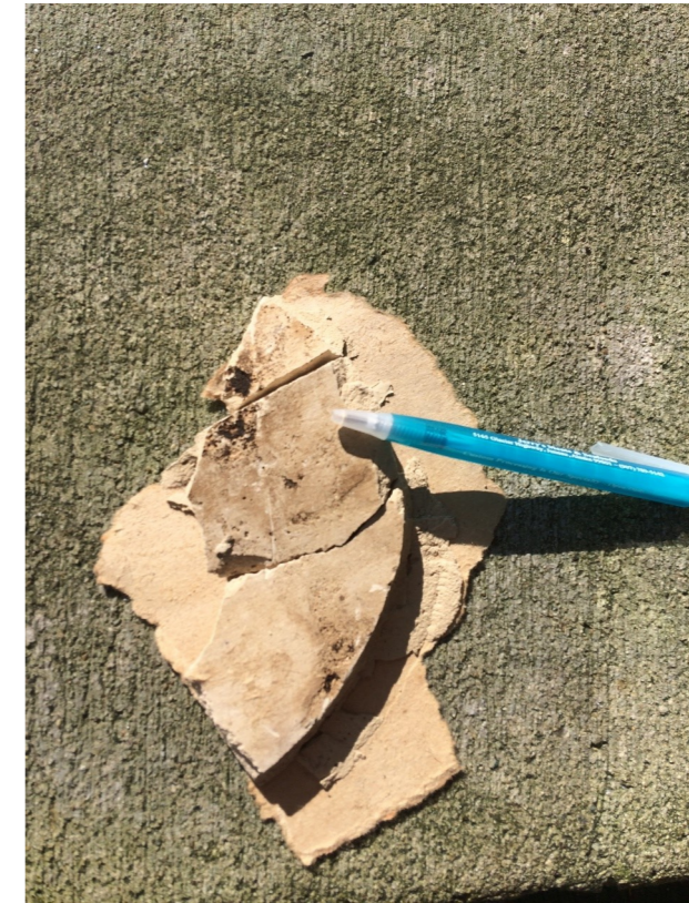
Back face of concrete board at removed area of Siding. Note remains of black mold where in contact With wet OSB substrate.
