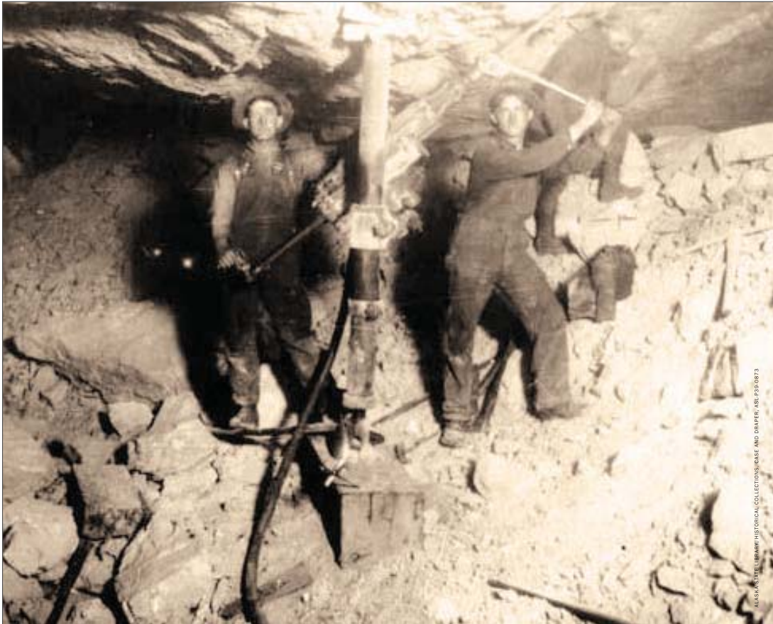
Underground lode mining in a Treadwell mine tunnel, 1908. The process was called Drill, Blast and Muck: miners first drilled holes in the rock with a large jack, and then packed it with explosives. After the blast, they mucked out the ore and sent it to the mill.
