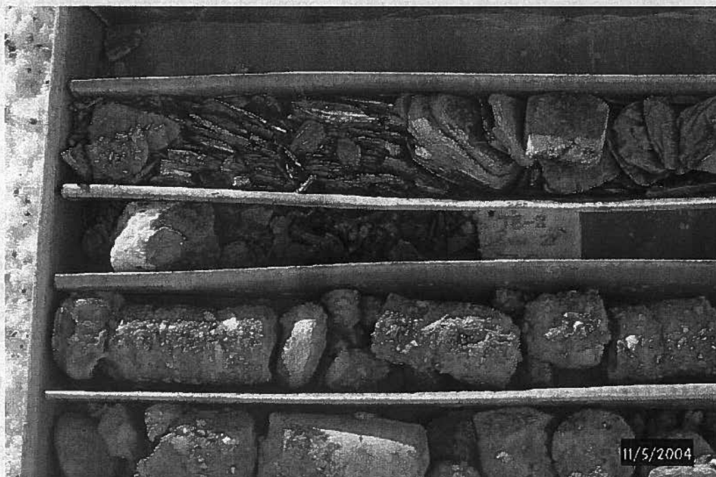
Photo 4. Core in the bottom of this photo is taken from within the till and the core in the top of the photo is from the weathered rock.
