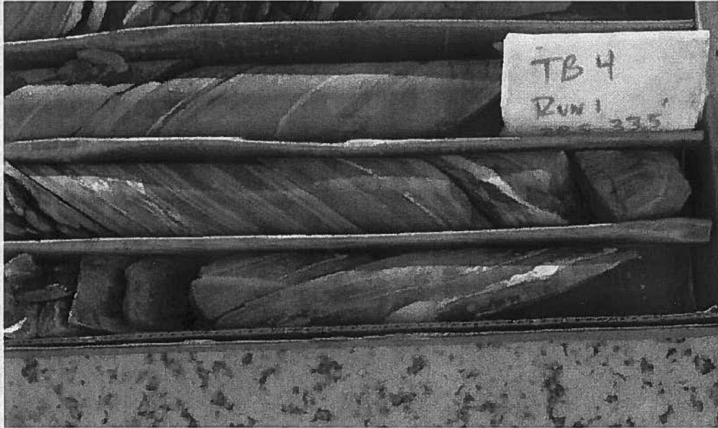
Photo 5. Rock core showing the steep angle of dip.
