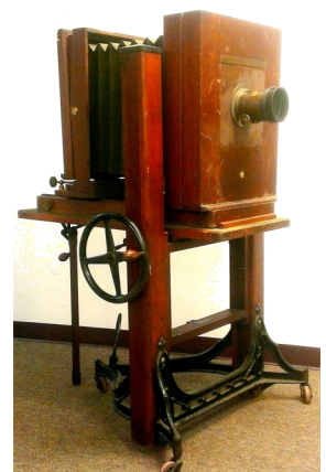
Kodak Century Studio Camera on a Kodak Semi-Centennial Stand, used by Winter & Pond. JDCM 2014.17.001
