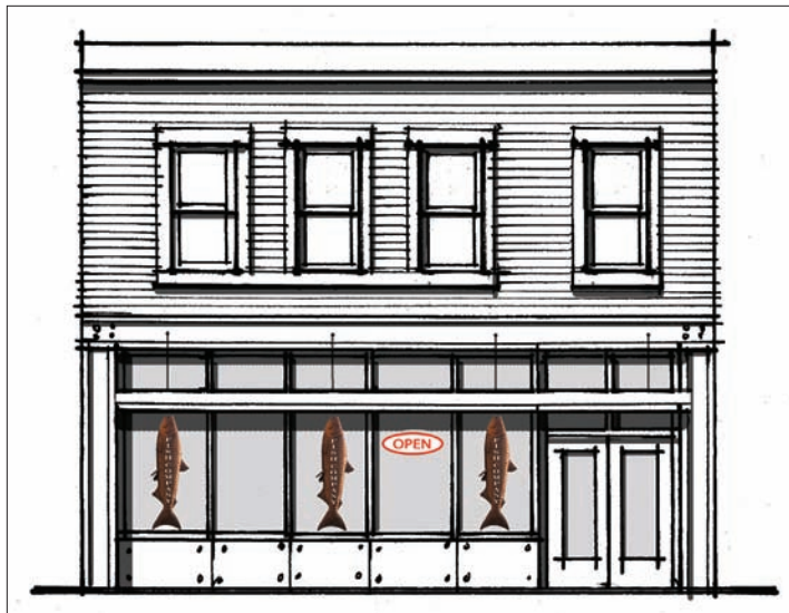
Window signs may be considered. The total window sign area should not exceed 10% of the total storefront glass (grayed area). The maximum window sign area is shown in this example
