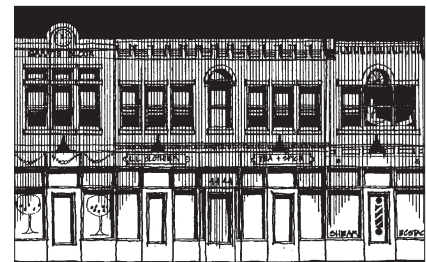
Prevent glare onto adjacent properties by using shielded and focused light sources that direct light onto the ground. The use of downlights, with the bulb fully enclosed within the shade, or step lights which direct light only to walkways, is strongly encouraged.
