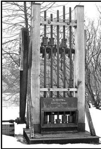
Five stamp mill restored in 2001 by CBJ Parks and Recreation staff.
