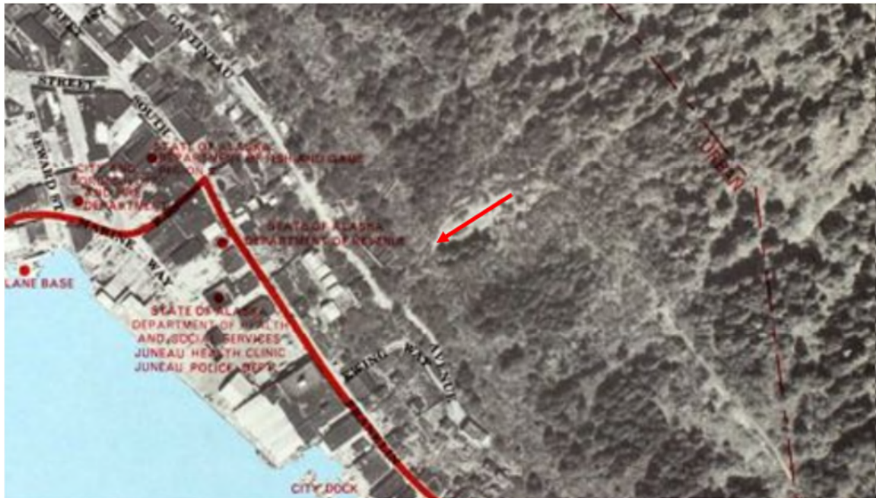
Figure 7: Excerpt from 1971 air photo mosaic showing a reactivated slope failure at the site of the 1936 landslide (red arrow). Since the 1968 air photo mosaic showed little exposed soil at this location, this slope might continue to slough and ravel periodically over time, confirmed by Tetra Tech’s mapping of mass movement features (Tetra Tech 2021a). (Image credit: Alaska State Library – Historical Collections, ASL- Map Case Juneau 1971 , ALS 2022e.)
