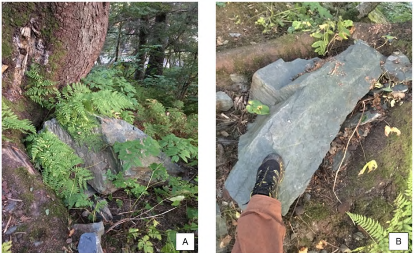
Figure 7: Photos from Tetra Tech’s main report, at the southwest end of Mt. Maria above Basin Road at Harris and 7 th Street. Photo P24 (Figure 7A) shows a tree damaged by rockfall. Photo P25 (Figure 7B) shows the typical size of some of the fallen rocks.
