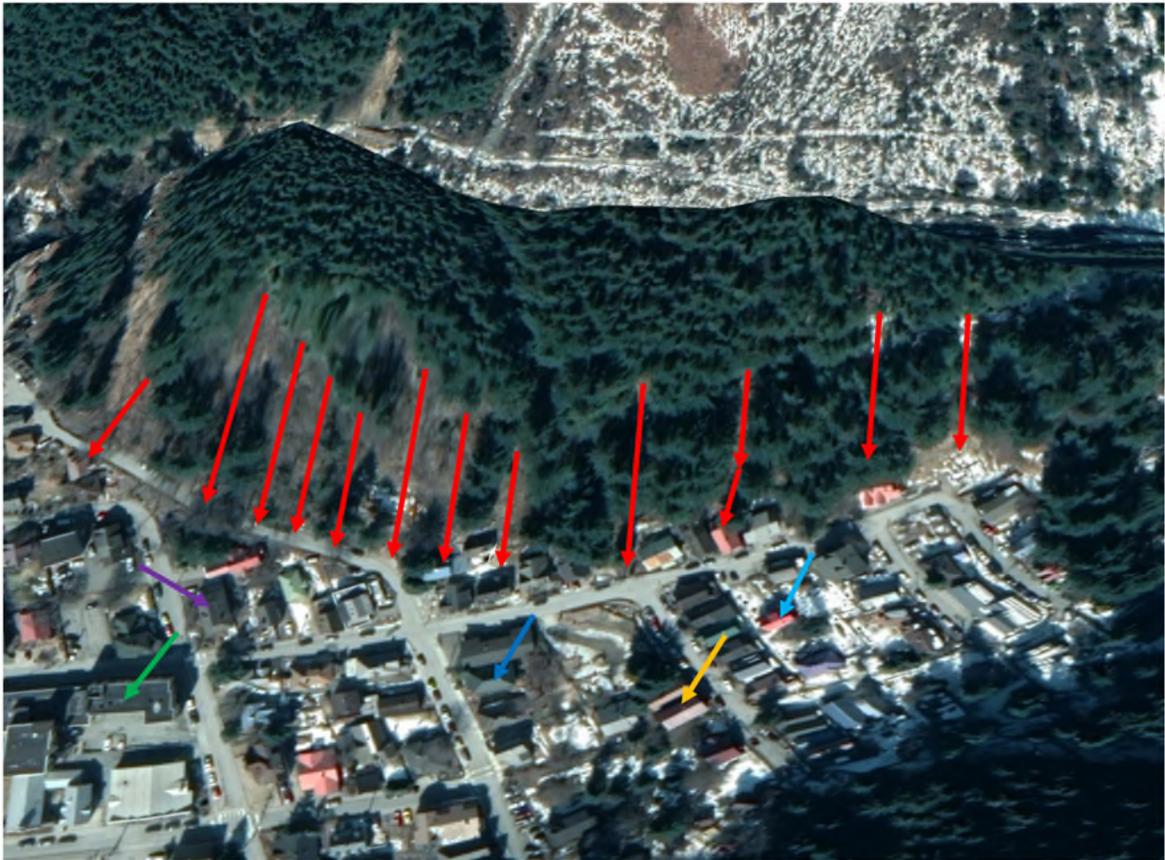
Figure 14: Looking north-northwest, this Google Earth view is from an eye elevation of about 1,100 feet in early spring (April 2020), so that the slopes currently lacking coniferous trees can be seen more easily. Several of the swales and slope sections lacking tree cover that were seen in the 1902 photo (Figure 13) are still visible in 2020, along with a few more slide paths (red arrows). The apparent alignment of the paths lacking trees is slightly different in Figures 13 and 14, due to the different perspectives of the images. The landmarks in Figure 14 are the same as those in Figure 12. (Image credit: Google Earth 2022.)
