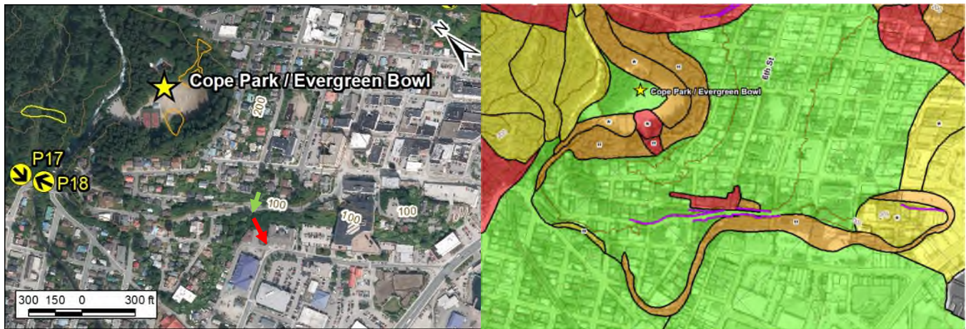
Figure 6: Excerpts from Figure 1.4b Slope Movement Features and Figure 1.6c Landslide Hazard Designation Mapping. On the left-hand image, the 1923 landslide is shown running downslope from Calhoun Avenue and the southeast end of Dixon Street to a little above the present-day Willoughby Avenue (red arrow). Landslides still occur at Calhoun Avenue, originating upslope of Dixon Street (green arrow). On the right-hand image, the hazard mapping from 1987 has been restored and updated above Calhoun Avenue, based on the debris slides reported by CBJ.
