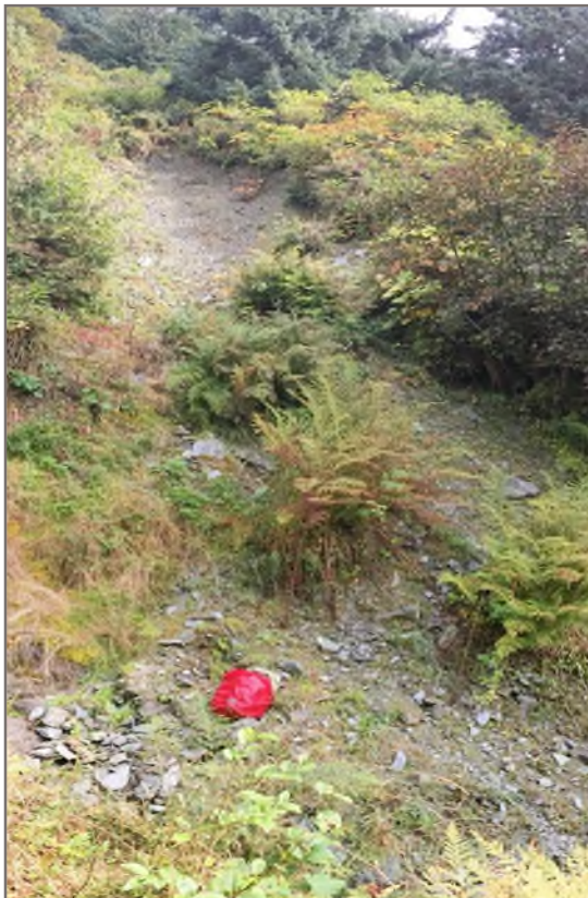
Photo 2: Looking east at a small debris slide within the White avalanche path. The bare ground near the top of the photo represents the initiation zone. The red backpack is resting on the deposited material consisting of platy schist cobbles/pebbles, sand, and silt (Date of Photo: September 11, 2019; The photo location is shown on Figures 1.4 and 1.5).
