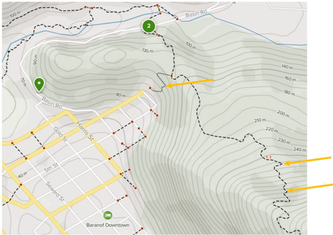
Figure 2: Topographic map, showing the same trail alignments as the pale gray lines on Figure 1. Dotted trail above Nelson Street is the trail section officially no longer used. Note switchbacks. (Image credit: AllTrails 2022).
