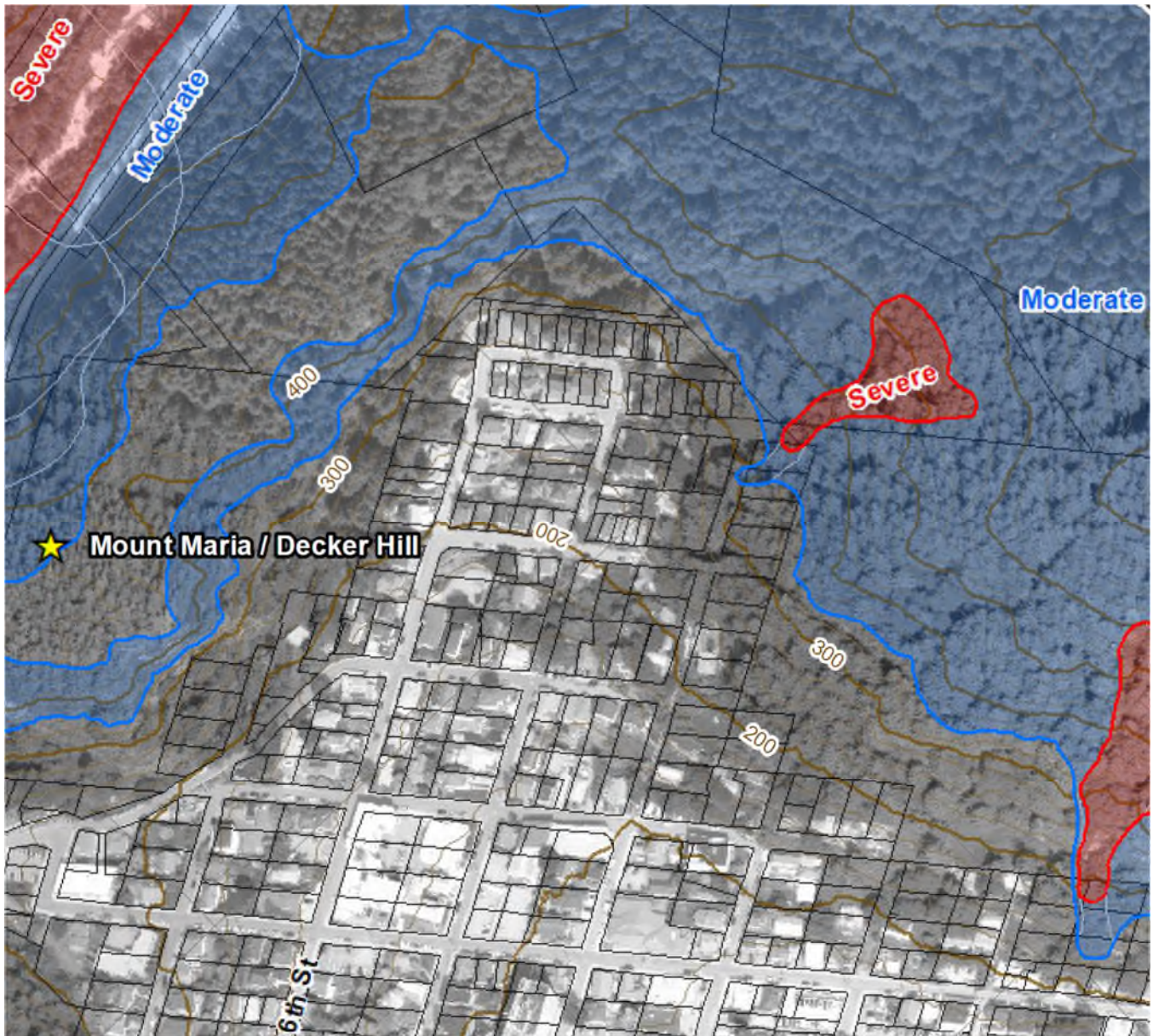
Figure 1: Excerpt from Figures 2.4c and 2.4h in the main report, showing the northeast end of the Starr Hill subdivision. Almost all of the lots are mapped with an avalanche hazard designation of Low (i.e., not colored as red or blue), with the only encroachment being the G000 (Park) avalanche path on the right (marked Severe , with Moderate terrain below). All the existing houses are currently located in areas designated as Low .
