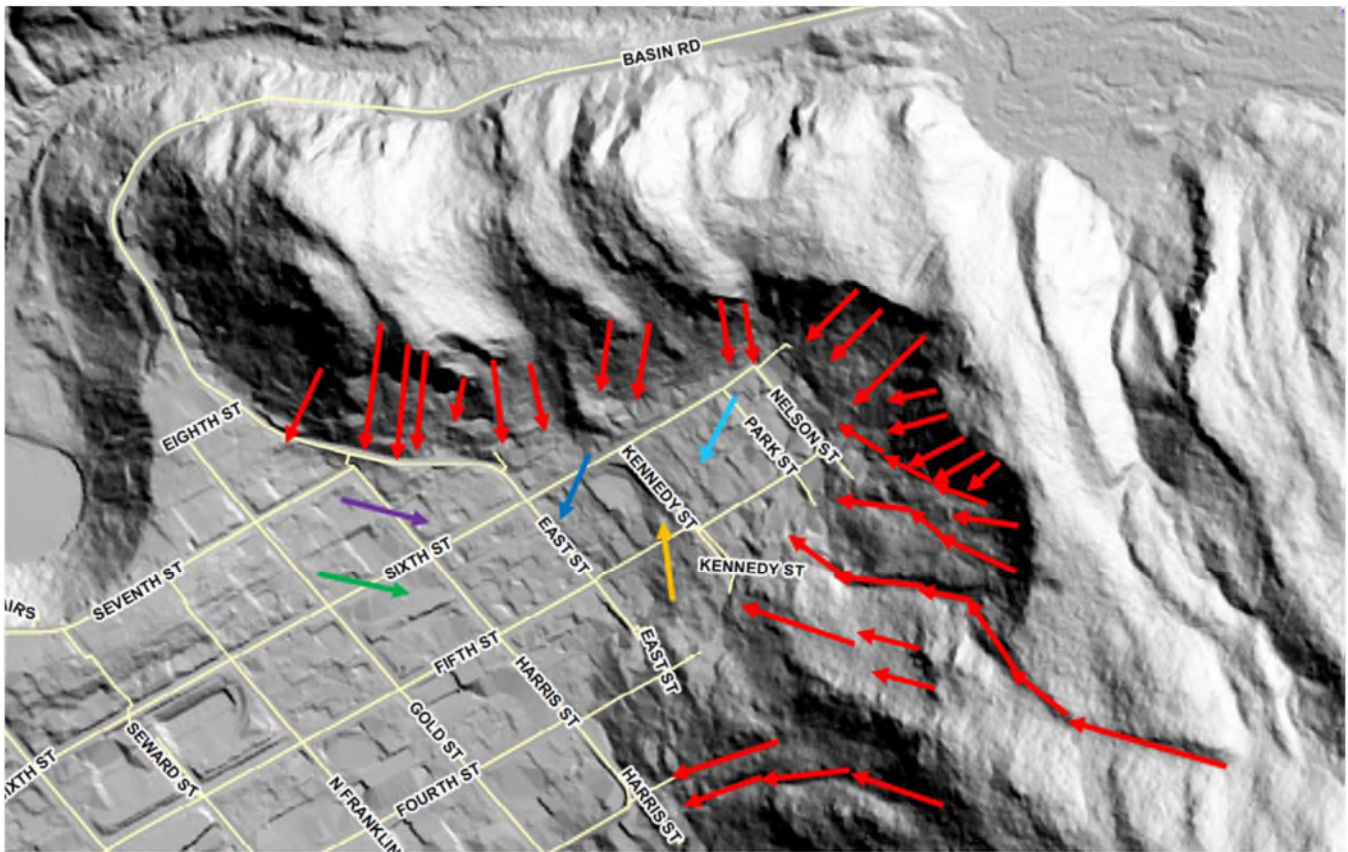
Figure 15: This excerpt from the 2013 LiDAR image shows several bedrock cliffs and bluffs above Basin Road, 6 th Street, Nelson Street, and the north end of 5 th Street. Fieldwork identified numerous active rockfalls/rockslides as well as some debris slide areas that confirm the observations from the LiDAR and the air photo mapping (Figures 6, 7, and 8). Apparent landslide locations shown are based on poorly-vegetated slopes, swales and gullies seen on Google Earth that are also visible on LiDAR hillshade models (red arrows). Landmarks are as for Figure 14. (Image credit: CBJ 2013.)
