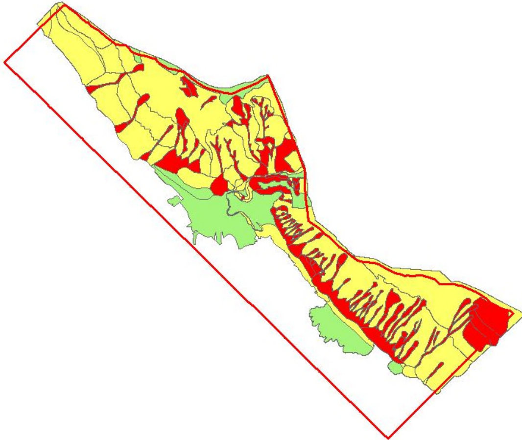
Figure B.5: Initial Landslide Hazard Designation Map. (Red = Severe, Yellow = Moderate, and Green = Low hazard)
