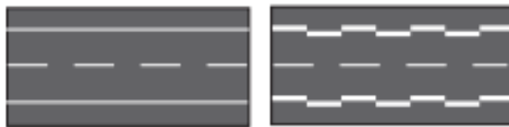
Examples of vehicle surface markings; roadways bounded by “zipper” markings are also used by aircraft.
