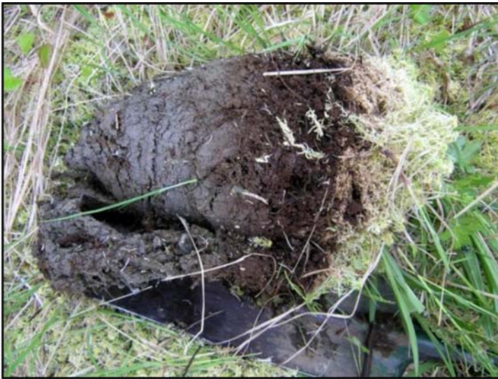
Figure 8 - Young wetland soil typical for Industrial Blvd project area. Saturated Sphagnum peat over uplifted intertidal silt.
