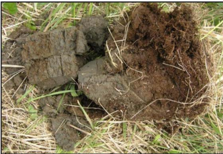
Figure 9 - Soil typical to upland areas in the Industrial Blvd project area. Unsaturated organic material and loamy soil over uplifted intertidal silt.
