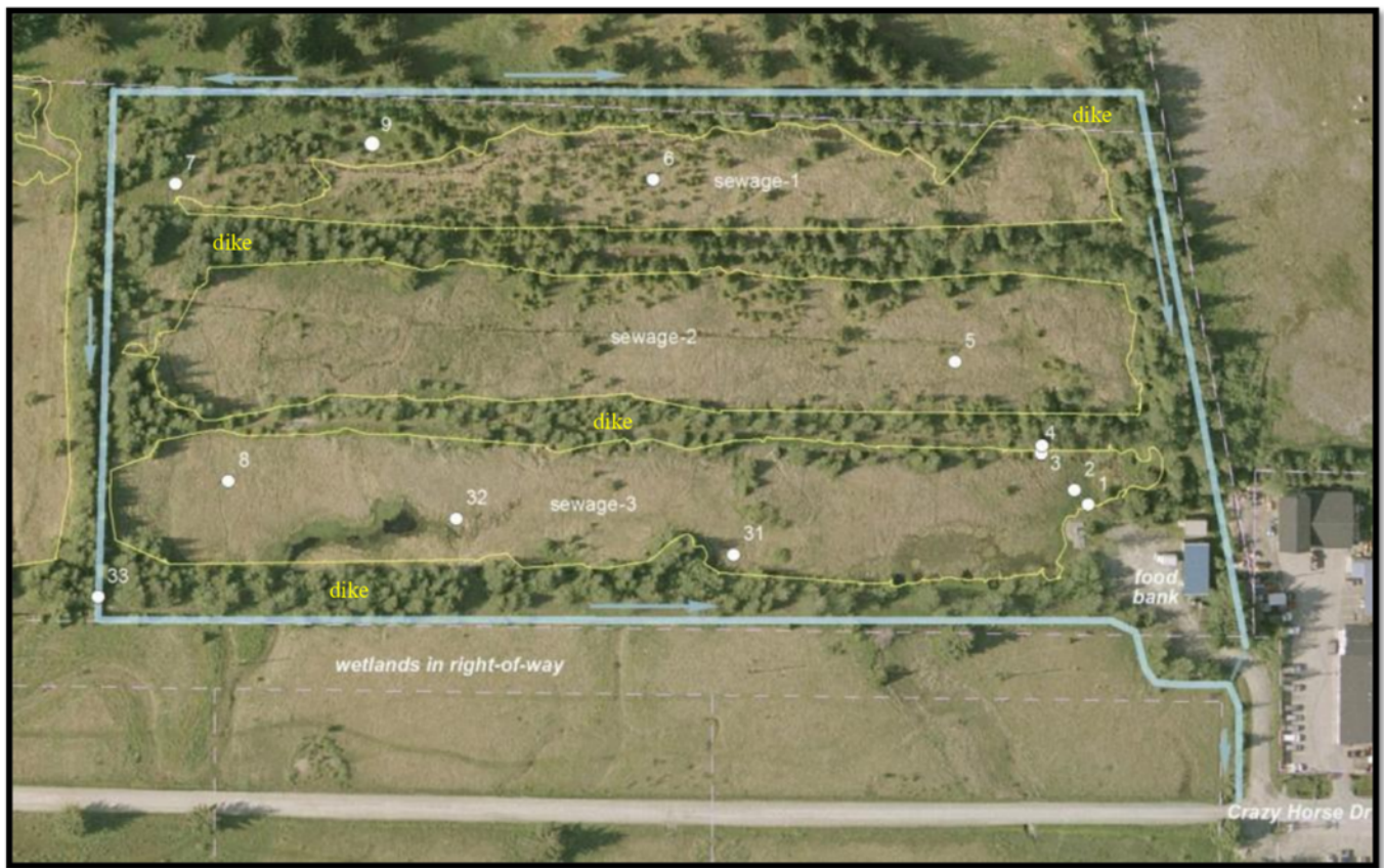
Figure 40 - Detail for sewage sludge disposal area. The blue-grey lines around the outside of the dikes indicate the ditch.
