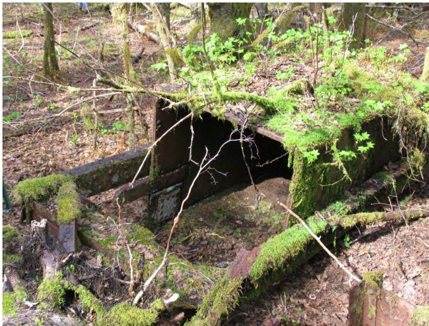
Skip at Central Hoist Shaft used to lift ore from Mine to Central Crushing Plant
