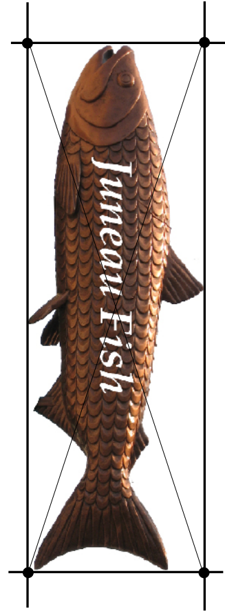
An irregularly shaped sign area is calculated by a simple geometrical shape juxtaposed on the object.
