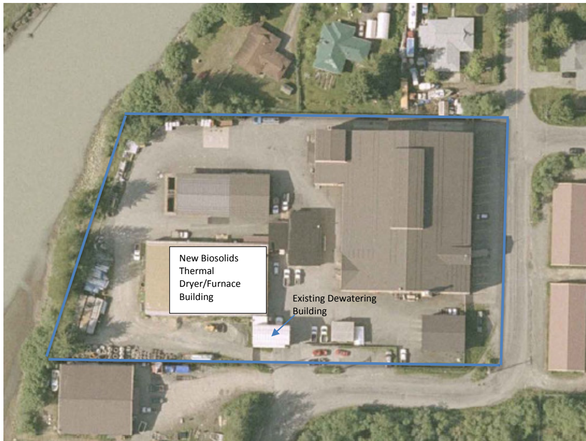
FIGURE 8 Potential Location of Thermal Dryer with Energy Recovery Furnace at the MWWTP Site
