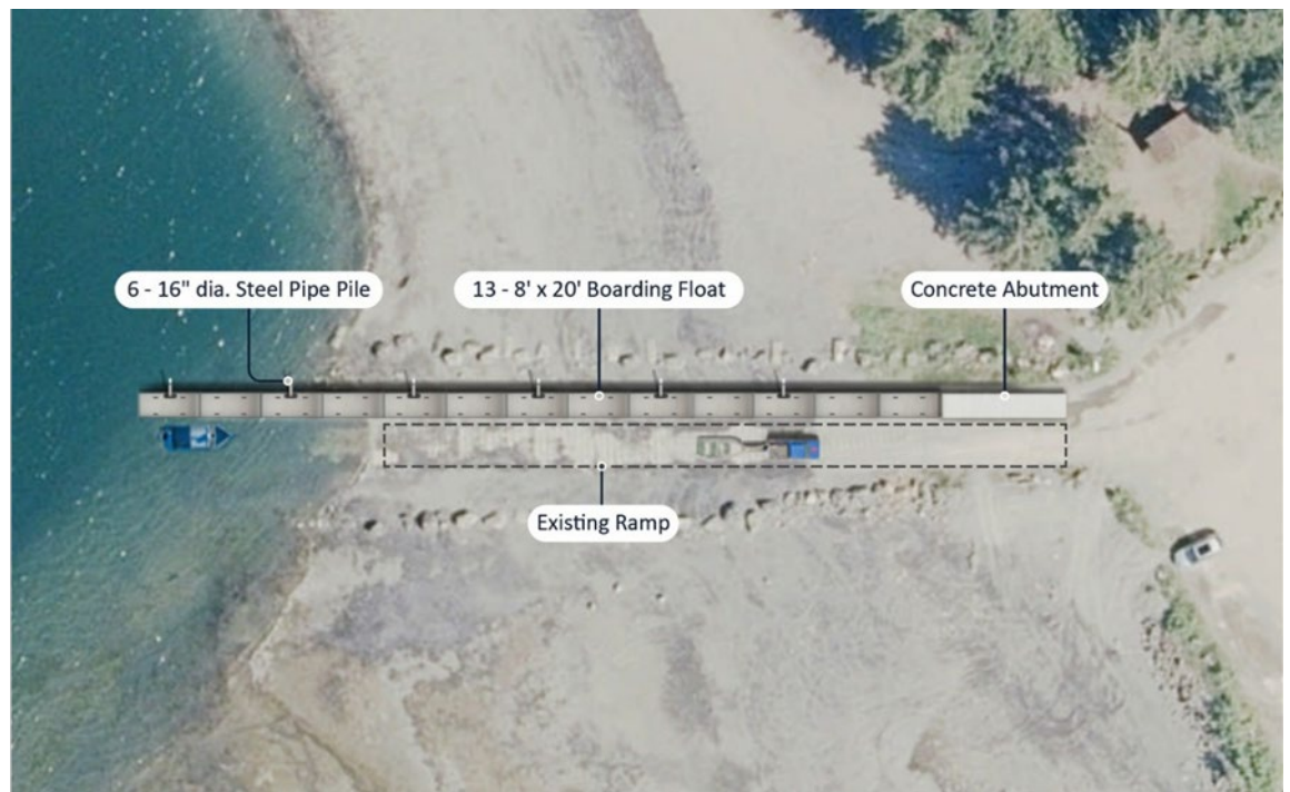
Proposed Boarding Float System (at Low Tide)
