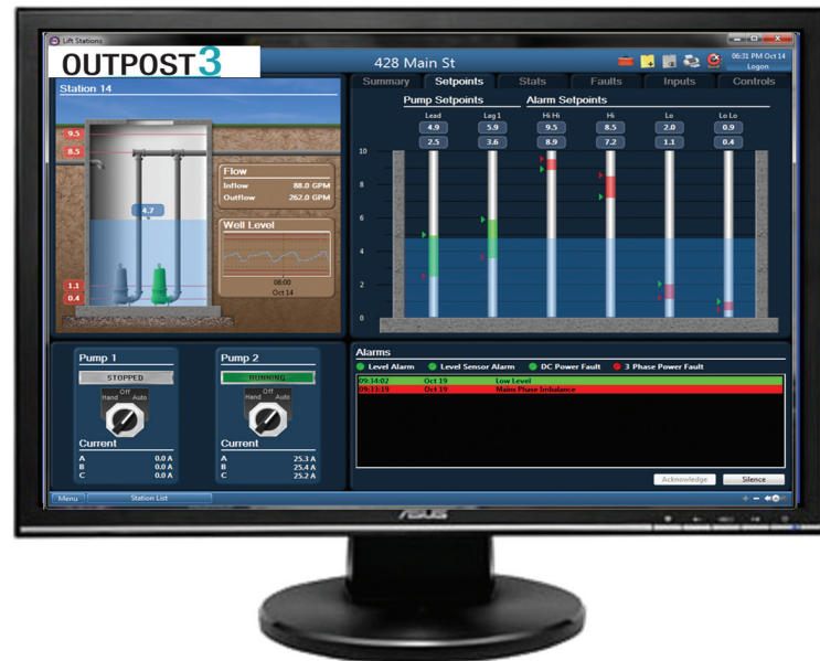
Remote pump control screen with MultiSmart and OutPost3 SCADA or PumpView3 hosted SCADA
